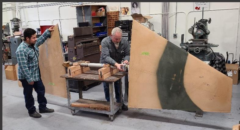
F-5 Horizontal Stabilizers Overhaul/Repair
